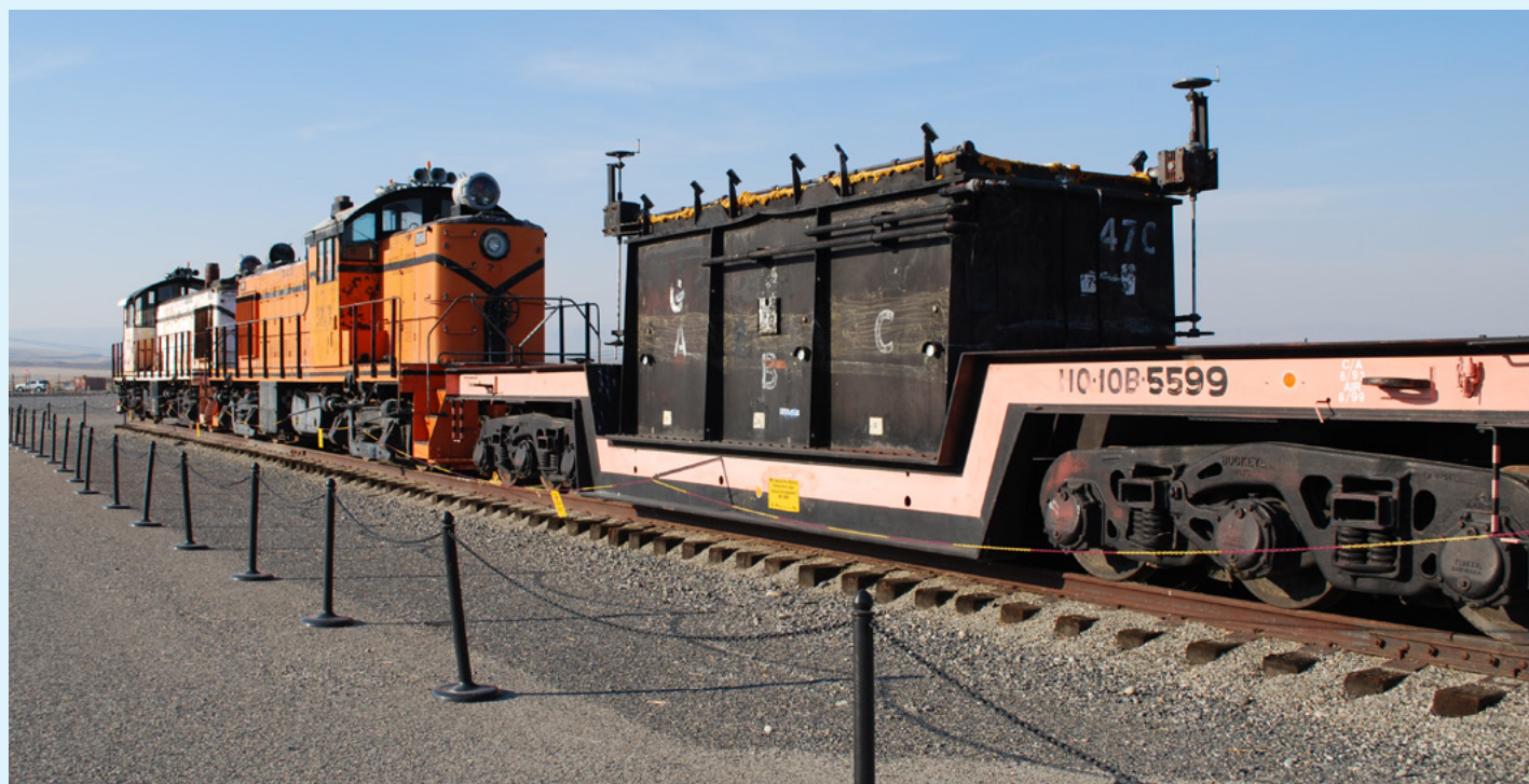
A cask car used to transport irradiated fuel from the B Reactor to the T Plant
